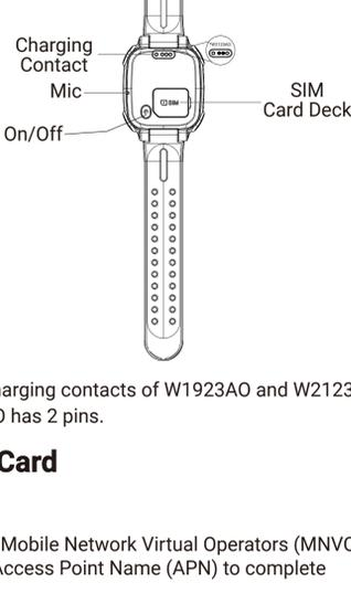
\*Remark: There is a difference between the charging contacts of W1923AO and W2123AO. The W1923AO has 4 pins while the W2123AO has 2 pins.
